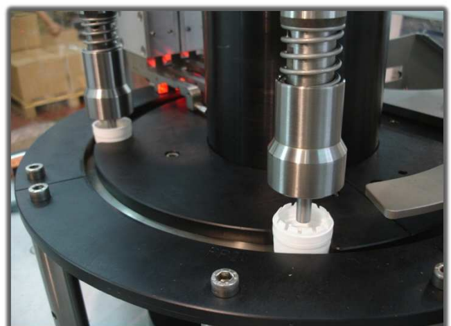
Example of folding machine CVA-041 for pharmaceutical cap
