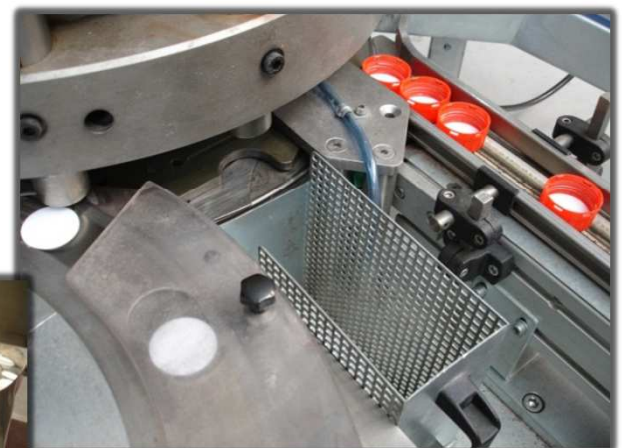
Example of insertion machine CVJ-122 for agro-chemical cap
