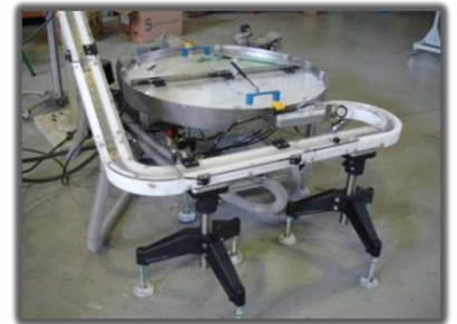
AC-101 Jet-air stream with accumulation turn table for caps at 100.000 cph
