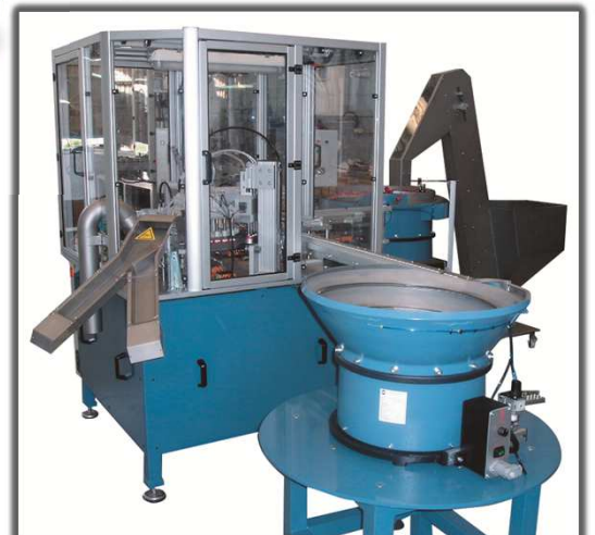
CIP-081 indexed machine 2 oriented components vinegar cap at 10,000 cph
