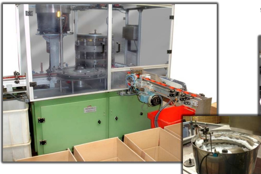
Example of insertion machine CVJ-122 for agro-chemical cap
