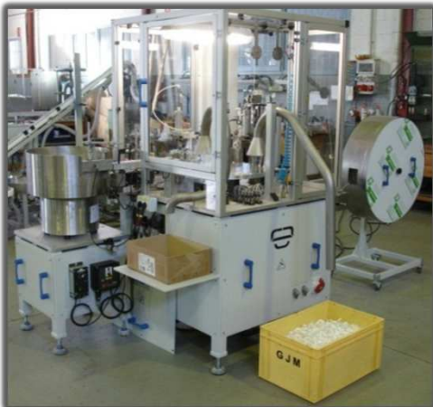
CIP-121 indexed assembling and testing machine for ophthalmic dripper at 3,000 pph
