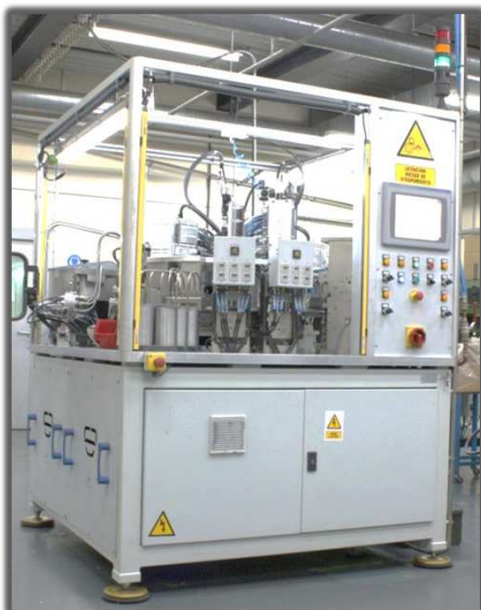
CIP-166 indexed assembly and leak testing machine for lighter at 16,000 pph
